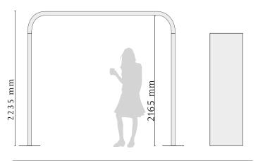
5 mm (0.2") foot + 1900 mm (74.8") screen + 330 mm (13"). Height: 2235 mm (88") from floor to the top of Arc. Inner dimensions from floor to ceiling of Arc is 2165 mm (85.2").
